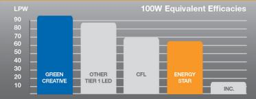
At 97 LPW, this lamp's efficacy is 10% higher than the Tier 1 LED A21 100W replacement industry average and exceeds new ENERGY STAR requirements by upwards of 50%. This energysaving performance makes this lamp a smart retrofit choice for incandescent and CFL bulbs.
